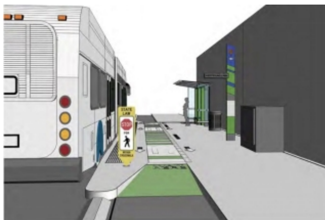
Figure 3. Illustration of a typical ‘bus boarder’ 2 .
